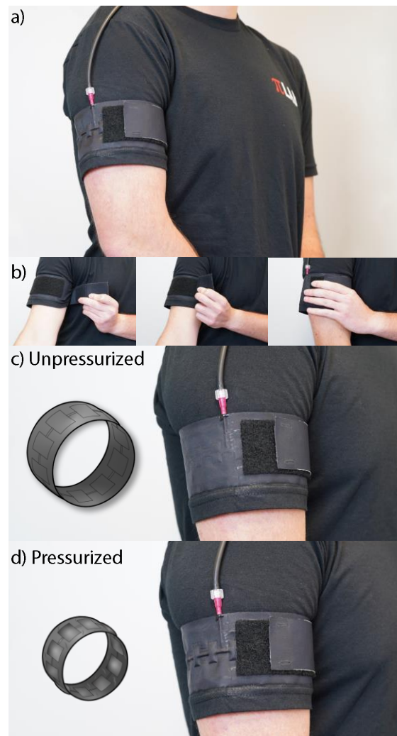
Figure 6. Seamless integration of a textile-based haptic device into a garment. (a) Shirt with a squeeze-enabled haptic device permanently heat sealed onto the sleeve. (b) Hook and loop fastening method to tighten the sleeve around the arm for a salient cue. (c) Unpressurized squeeze band on arm. (d) Squeeze cue delivered through application of pressurized air.
